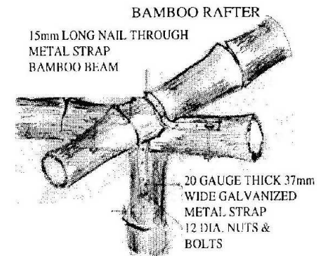
FIXING DETAILS BETWEEN POST, BEAM &amp; RAFTER
